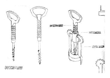
Fig. 6. Corkscrew disassembled and represented.
